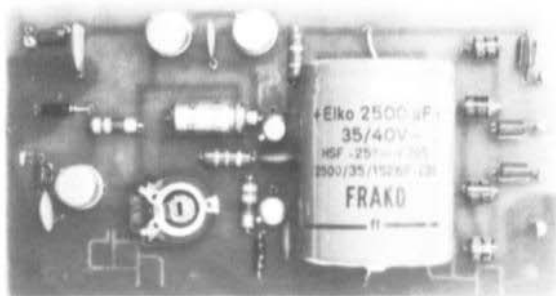
Fig. 5: Photograph of the stabilized power supply
